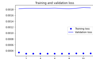
Fig 3 b) Encoder-Decoder LSTM Training and Validation Loss
