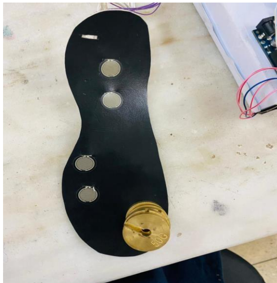
Figure 6. Calibration using known weights
