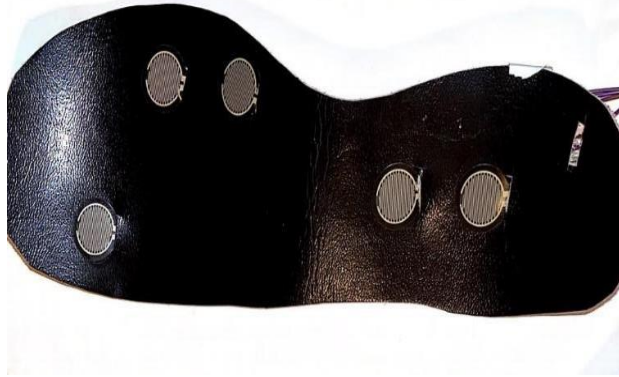
Figure 1b. Placement of FSR
