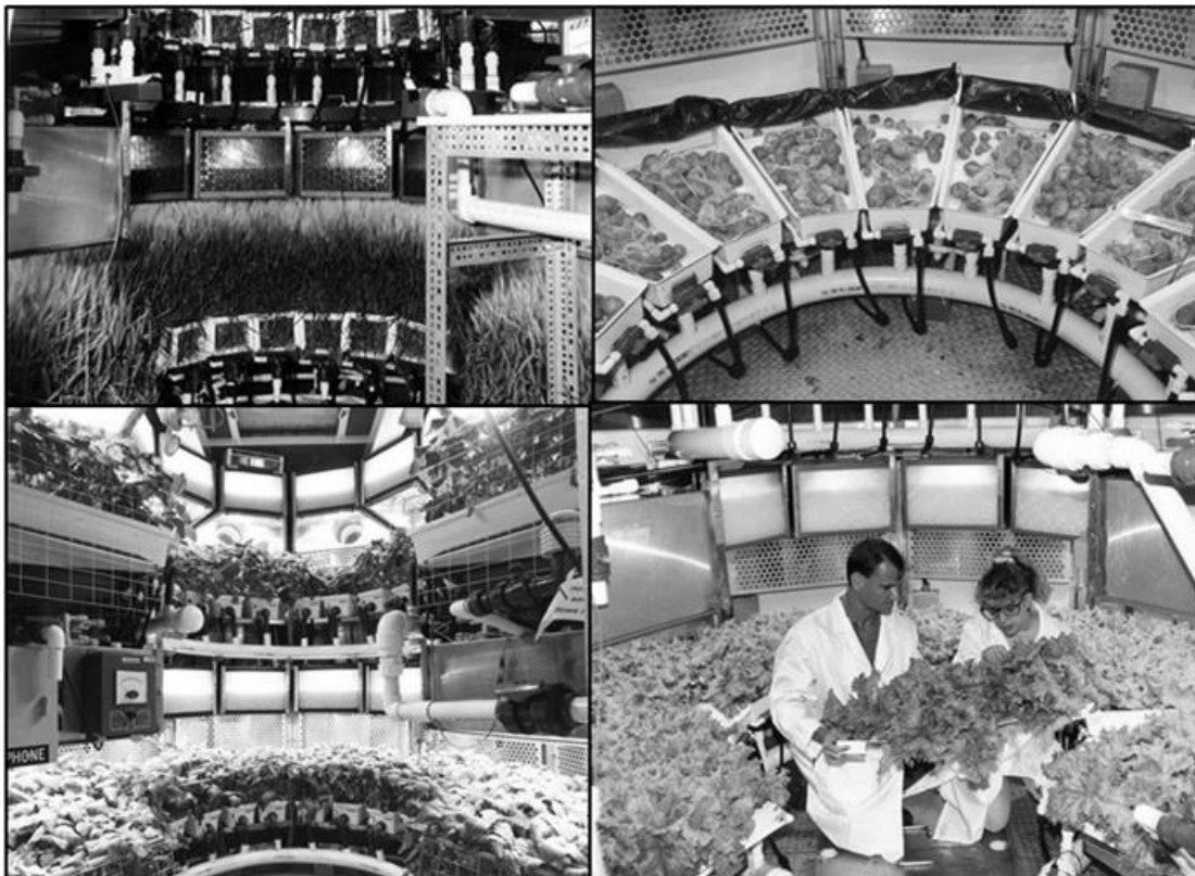
Figure 8. Internal views of the BPC showing the light banks and shelves, hydroponic trays and supporting plumbing. a) Upper left: wheat; b) Upper right; potato, with tray tops removed; c) Lower left: soybean; d) Lower right: Lettuce. Credits: NASA
