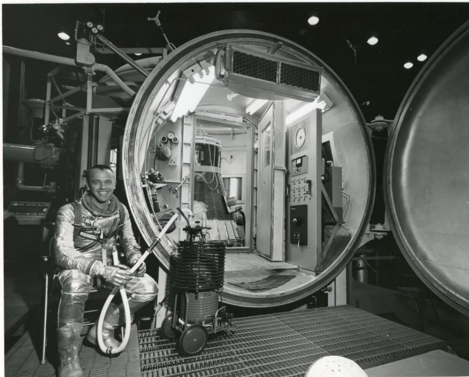
Figure 2. Astronaut Alan B. Shepherd, Jr. with the Mercury Altitude Chamber containing the Freedom 7 spacecraft. Credits: NASA
