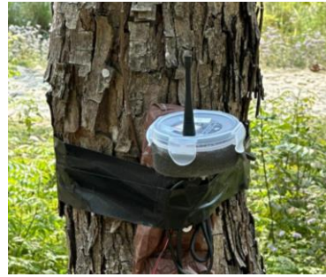
Figure 2. A CARACAL acoustic recording device deployed in the Dalla community forest.
