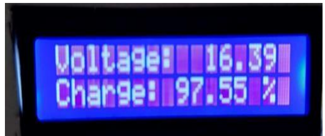
Figure 8: Car battery percentage & voltage on LCD Display
