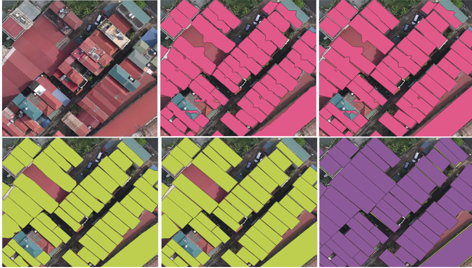
Fig. 4: The first top-left image is the input image, second and third is the Mask R-CNN predictions and geometry correction algorithm predictions respectively. The first lower-left image and second are the Multi-model predictions and corresponding geometry correction algorithm predictions, and the third image is the expected output image.
