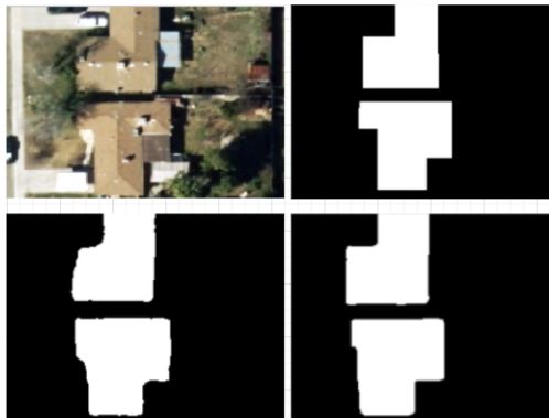
Fig. 2: Top left: Input image. Top right: Ground truth mask. Lower left: Mask was predicted by Mask-RCNN model. Lower right: Mask was predicted by multi-model (Mask-RCNN model combined with U2-net model).
