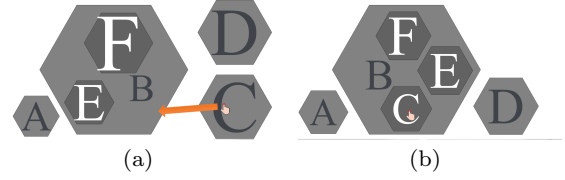
Fig. 10: moving node C from the child node of root to node B. (a) before modification, (b) after modification.
