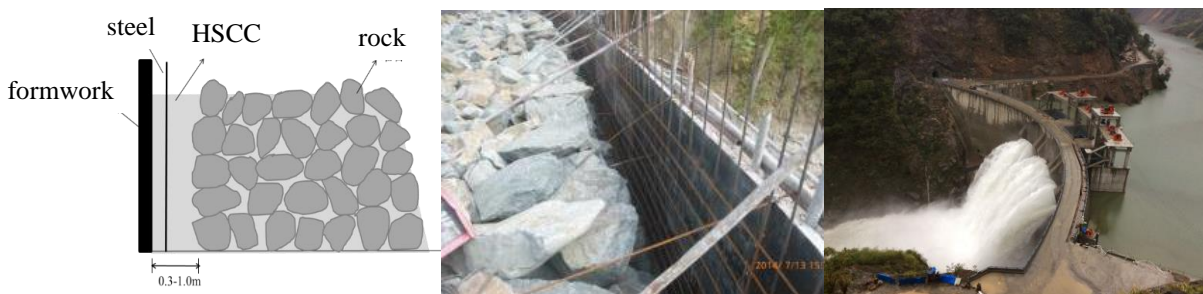
Figure 7: Structure, photo of integrated impermeable layer and Baijia RFC arch dam (H = 69 m)
