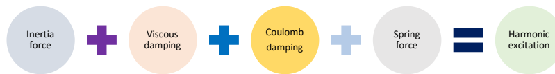
Fig. 2. Elementary expression of mass, damper, spring dynamic system subject to harmonic excitation for stick-slip friction rheology in bio-inspired tribology (a) Inertia force is a function of mass and acceleration (b) Viscous damping for environmental sound generation (c) Coulomb damping for frictional energy loss (b) Spring carried an expression of elasticity (d) The driving force is termed harmonic excitation
